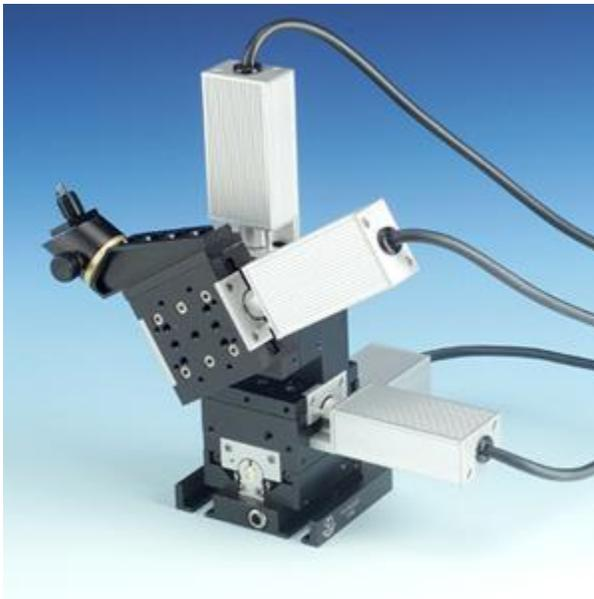
*Figure 4. Higher performance micromanipulators provide automated (pushbutton/software) positional control by using incorporating electronic actuators. This MX7600 system from Siskiyou is based on DC servos since these produce zero EMI when stationary, unlike piezos or microsteppers.*
