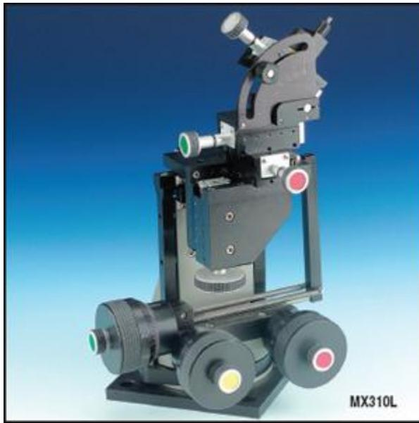
*Figure 2. Traditional Huxley-style mechanical micromanipulators are based on flexures and usually incorporate dial-like knobs for manual adjustment. This modular MX310L system from Siskiyou, coarse adjustment is provided by incorporating lower resolution stages at the top of the assembly, and simple pipette replacement is supported by a rotary stage at the base of the system with a hard mechanical reference stop.*
