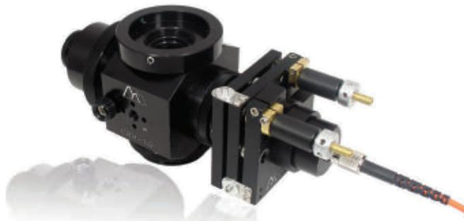
**FIGURE 2.** The IS-OGP is a modular sub-assembly from Siskiyou that collimates light from an input single-mode fiber and directs it anywhere in the field of view of an upright microscope via a 45° beamsplitter. The resultant light spot has an adjustable diameter and can be precisely located or scanned via mechanical (differential screw) or automated actuators.
