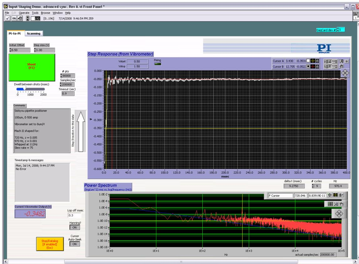
Figure 4. Same as Figure 3 but using Input Shaping<sup>®</sup>. The rapid actuation of the PZT no longer excites resonances in the structure and pipette. The cleaner step means repetitive switching is eliminated.
