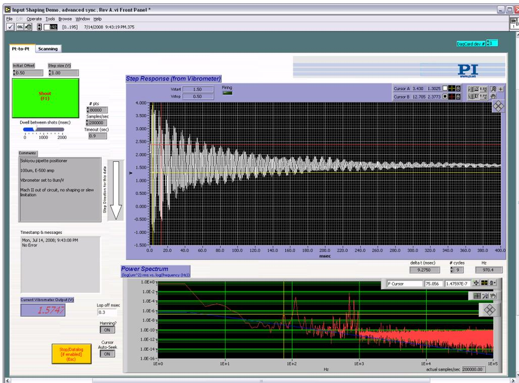
Figure 3. Interferometric position metrology of pipette motion using a laser Doppler vibrometer operating in the position domain. Top graph shows vibrometer position output in Volts ( $8V/\mu\text{m}$ ) vs. time after a sharp step *without* Input Shaping®. Motion-driven vibrations in the structure and pipette constitute ringing which can manifest as unwanted repetitive switching of the theta glass solutions.
