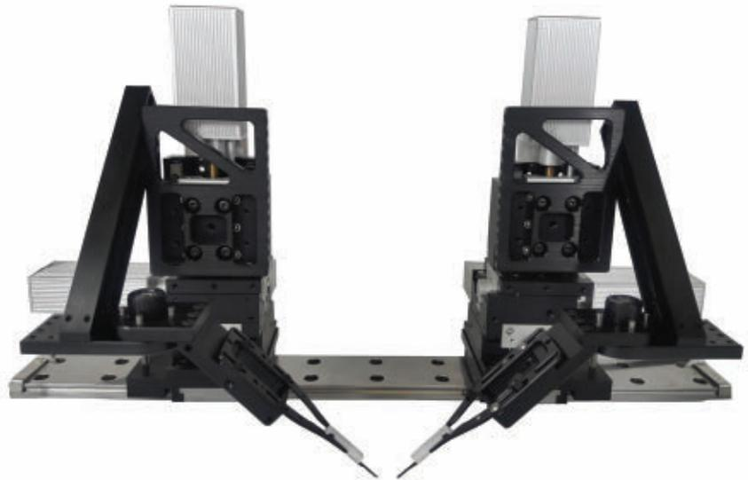
**Figure 4.** The inner workings of a MyoStretcher feature two tipped rods that can apply and/or sense minute forces associated with a single myocyte. The rods are positioned using DC servo units; Siskiyou MX7000 series. Courtesy of IonOptix.
